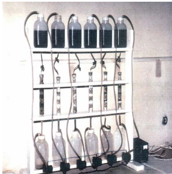
Figure 1: The glass percolator columns.
